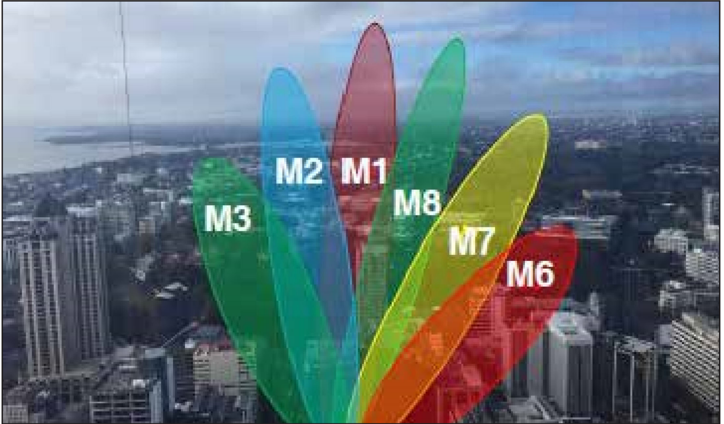
Fig. 5 • View from behind the 21 dB gain antenna system. 6 beams, M3 (left outermost beam), M2, M1, M8, M7 and M6 (right outermost beam).
