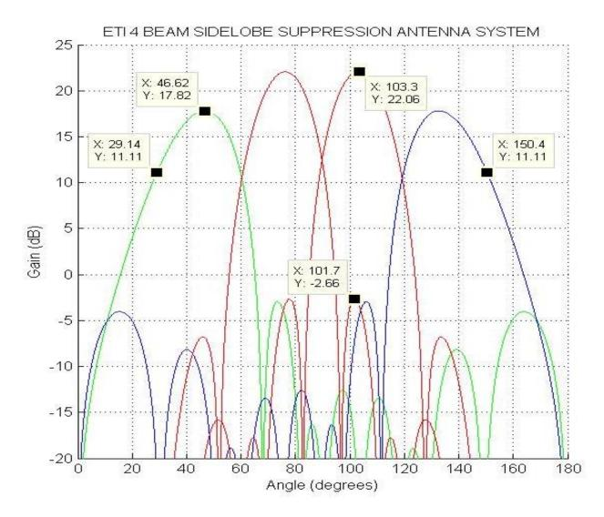
A Multibeam 120 degree Antenna System with beam crossover, maximizing signal to noise ratio. This Antenna System can be employed with a single channel repeated four times thus quadrupling the data throughput. Available on all Telecom bands.
