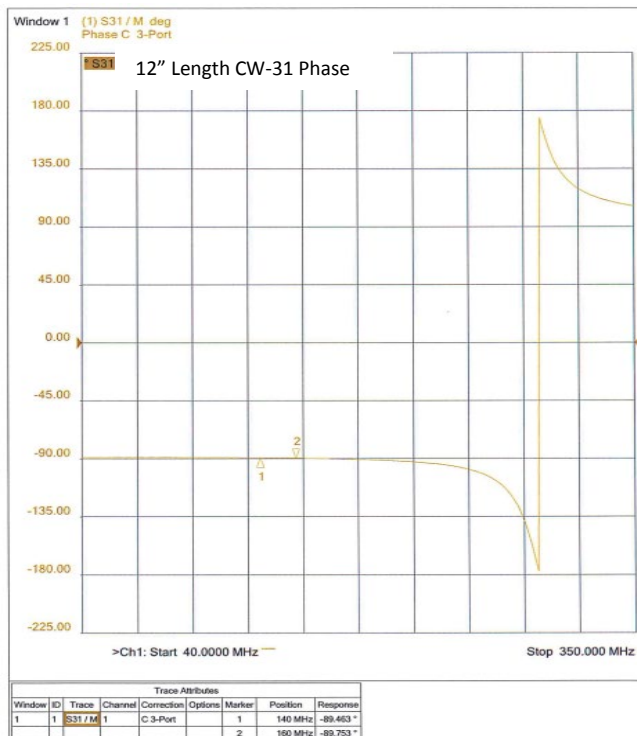
Figure 3: Phase at 160 MHz and 12.5" Length
