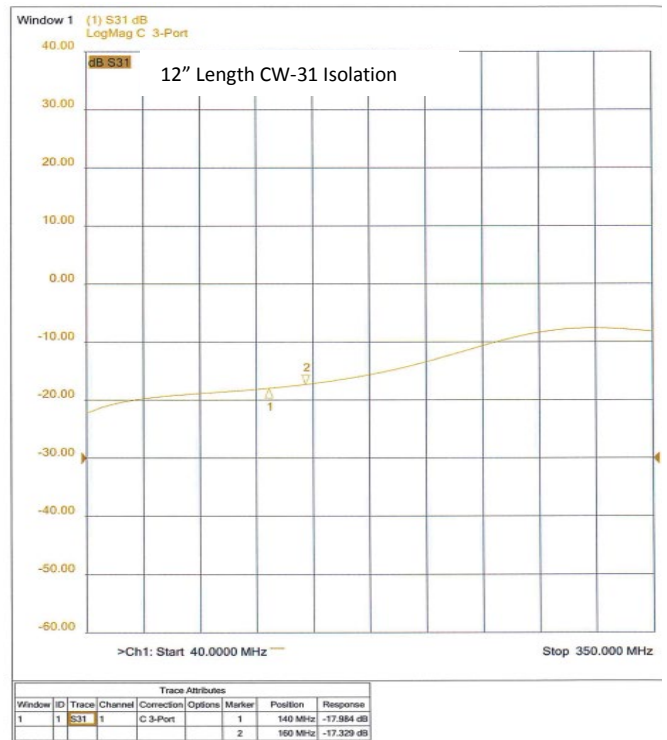
Figure 2: Isolation at 160 MHz and 12.5" Length
