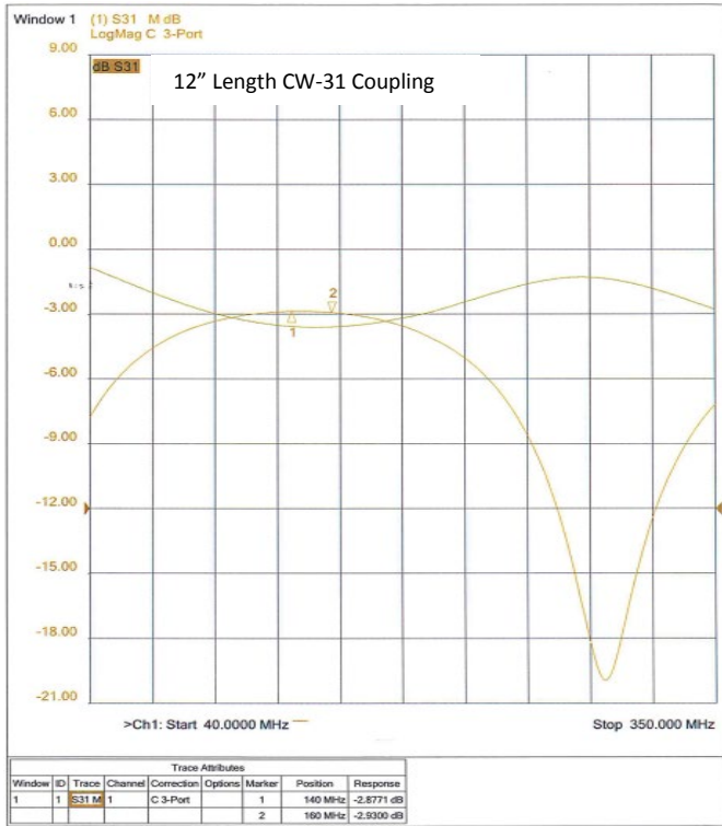
Figure 1: Coupling at 160 MHz and 12.5" Length
